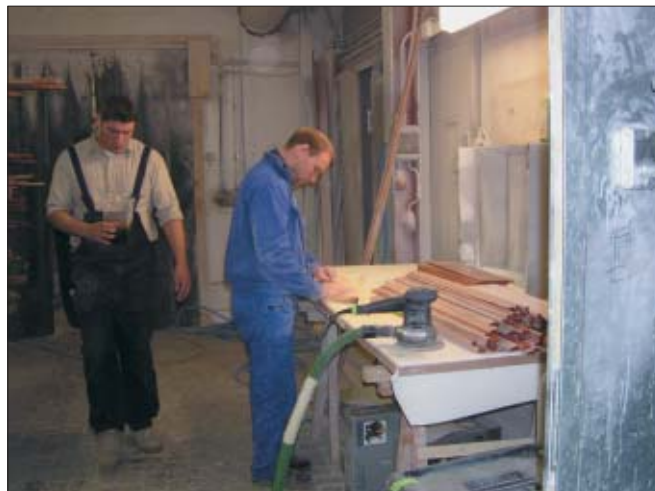
Left —Cabinets are readied in the carpentry shop before being installed. Right —A carpenter prepares stock for an interior component. Rounded-wood pieces are manually sanded.
