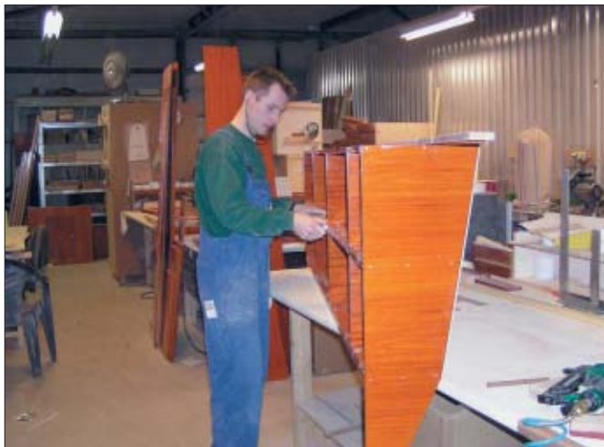
Left —Cabinets are readied in the carpentry shop before being installed. Right —A carpenter prepares stock for an interior component. Rounded-wood pieces are manually sanded.
