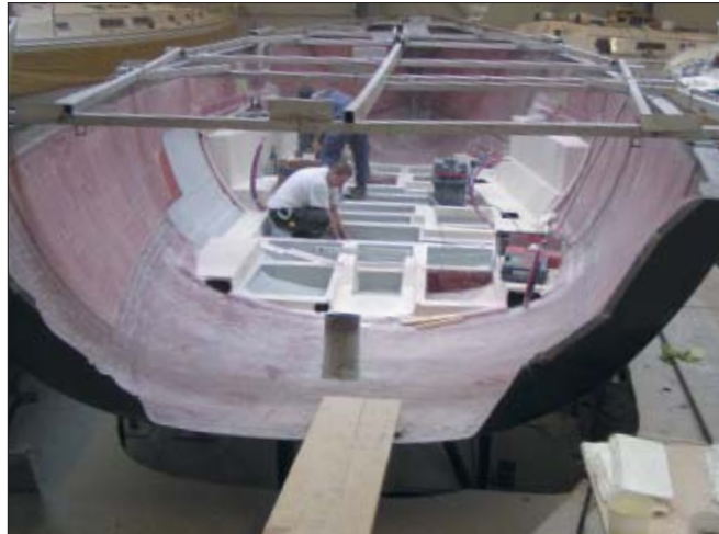
Left —Wood cabinet parts pass through the Rotoclean Cattinair spray varnish machine, on a conveyor belt. The same machine also dries the varnish. Right —An aluminum grid holds the hull shape while workers tab the grillage in place, which will be followed by bulkheads.
