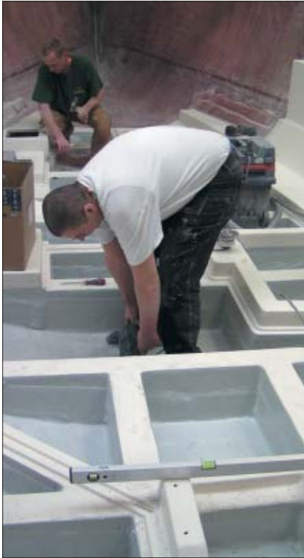
Left —A molded grillage tabbed to the hull stiffens the bottom. Right —Production manager Gregor Bredendeck.
