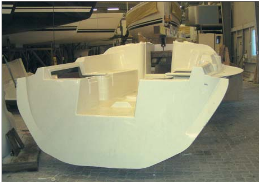
The deck mold incorporates a flanged transom. Its open design eliminates the expense and complication of scuppers, and caters to a decidedly performance-oriented clientele.
