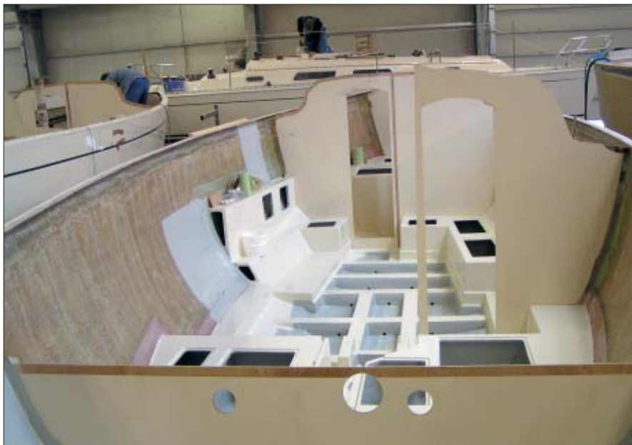
Hulls are laid up by hand. Bottoms receive solid glass; balsa or Airex cores are applied to the topsides only. Plywood bulkheads get tabbed to the hull. The 371 is shown here.
