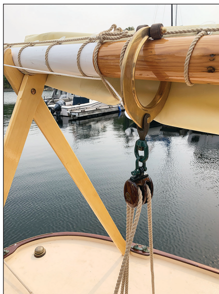
Far left —Lawson made a new tiller from a section of 1¼" bronze propeller shaft. The cap on the rudderstock reads "DOROTHY 1897." Left —Because the boom must rotate to reef the mainsail, the sheet is attached with a so-called reefing claw.
