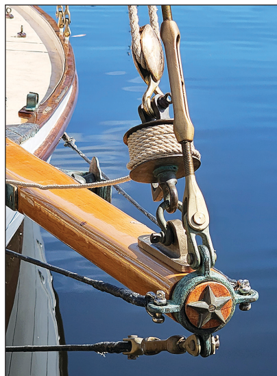
DOROTHY's jib is now managed by a relatively new Wykeham Martin furler whose parts are cast to original 1905 patterns.
